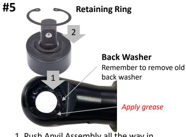
1. Push Anvil Assembly <u>all the way in</u> F/R lever can only be turned ~40 degree
