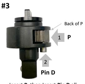
Insert **P**, then Insert **Pin D** <u>all</u> <u>the way in</u>
